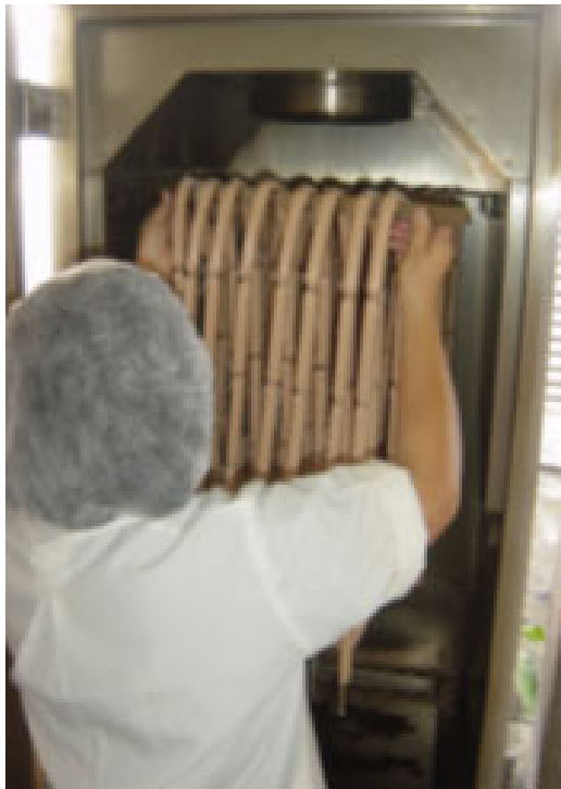
Fig. 69: Hotdogs are placed in the smokehouse for hot smoking (pale colour before smoking)
