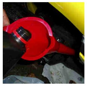
Place a funnel into the dip stick port and slowly pour in slightly less oil than the capacity stated in your owner's manual.
