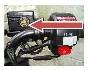
Next - there are 2 Philips head screws on the top of the little box. Remove the screws and carefully lift off the cover and set it away from the scooter. Carefully add a few drops of DOT 3 brake fluid at a time until it reaches the top of the sight glass. Replace cover and tighten both screws. Wipe the entire area around the cover with clean paper towels. That's it.
