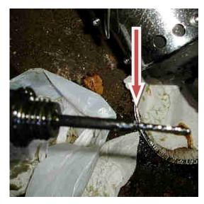
Wipe off the dip stick and Insert it into the hole but do not screw it in. Pull the dip stick out and check the oil level. It should be just at the top of the last tic mark.
