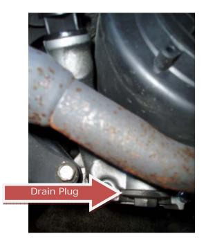
Place the shallow pan under the drain plug and loosen the drain plug using the 17mm wrench. Slip the wrench over the bolt head and pull from right to left to remove and drain the old oil. A spring and screen filter may also come out with the oil.
