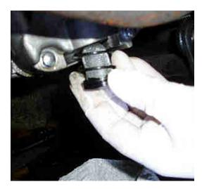
Replace the spring and screen filter and screw in the drain plug. The recommend torque is 20ft/lbs which is not much.
